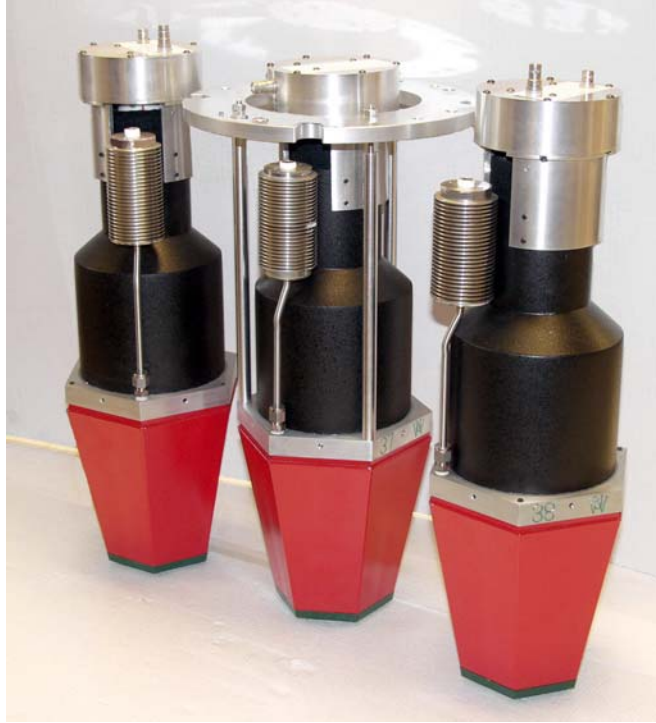
Fig. 2. A photograph showing three neutron detectors. The detector at the center shows the mounting ring that connects the detector to the GAMMASPHERE Al frame. Three stainless steel rods connect the detector flange to the coupling ring. The expansion bellows are seen with the plastic covers that normally protect the bellows removed.
